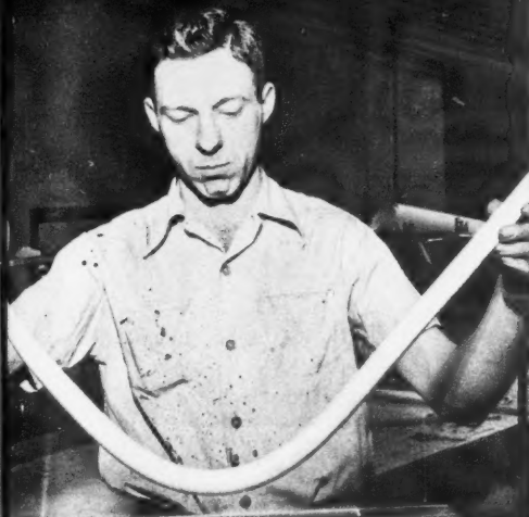
Before "blowing up" a neon sign, the glass worker, top, bends straight tubing over a wide gas burner.
